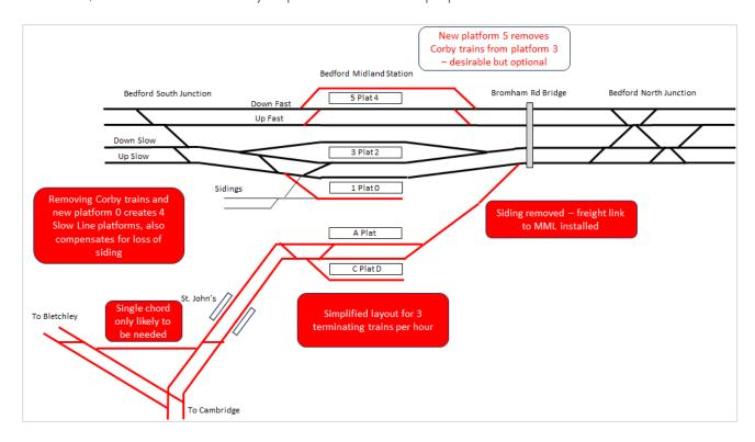
Figure 23 - Alternative Bedford layout for South of Bedford alignment service pattern - Option 2
