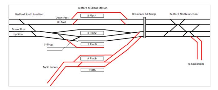
Figure 20 - Four-track option used for EWR Co's modelling
