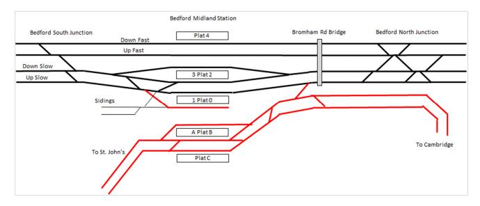
Figure 21 - Six-track option used for EWR Co's modelling
