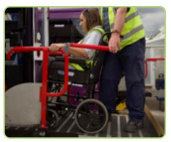
• Do not attempt to get off the lift until the backstop is fully deployed .
