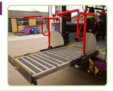
Having removed the passenger and wheelchair restraints, a team member manoeuvres the wheelchair from its travelling position so that the rear wheels are lined up to the edge of the lift platform.
