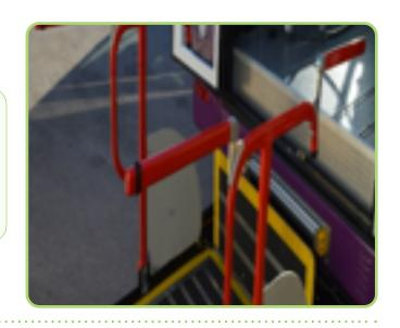
A team member operates the lift from outside the vehicle, ensuring it is fully deployed and the guard rails are fully extended.
