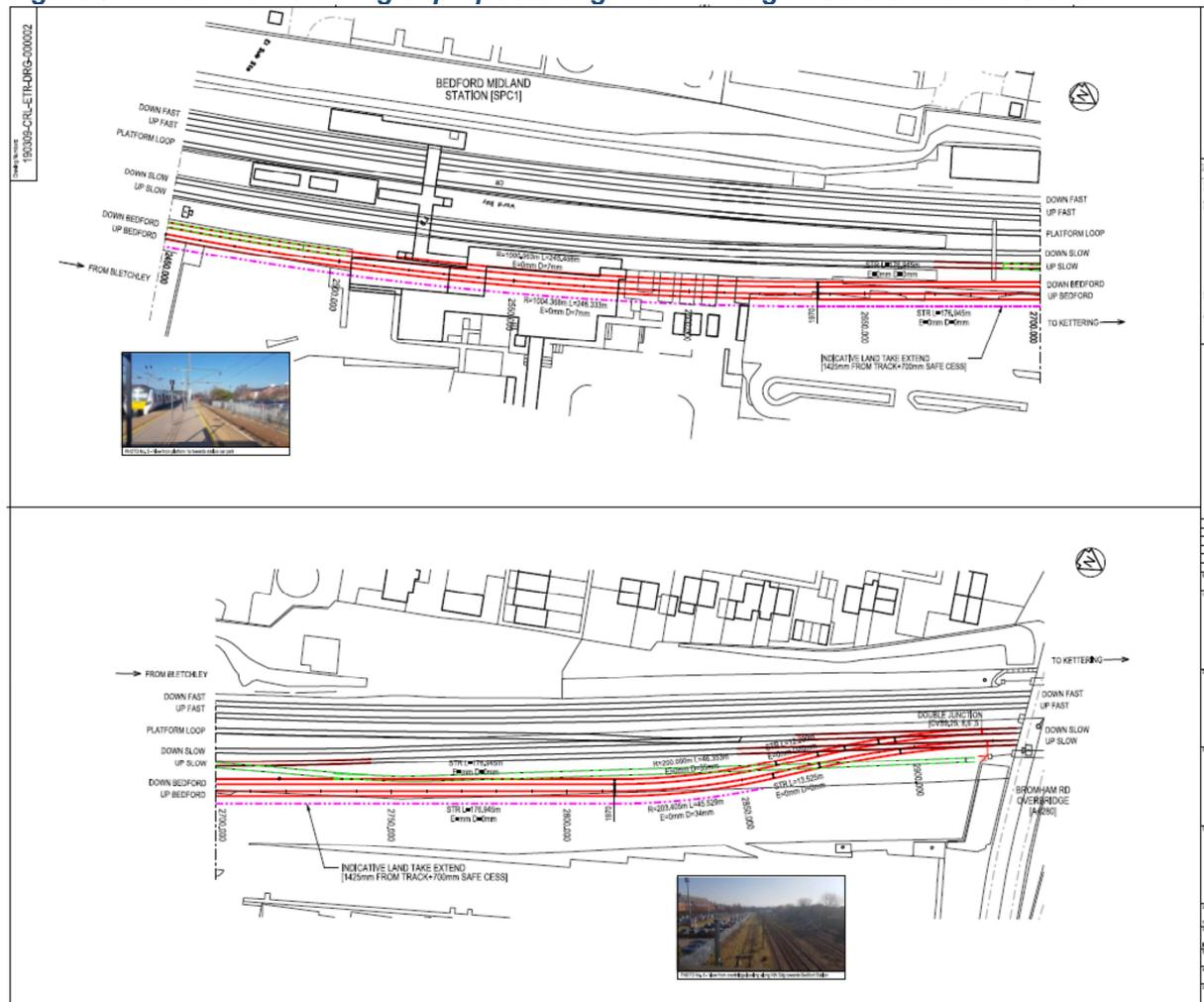
To the north of the platform, the tracks straighten up to run alongside the Slow lines on the bed of the existing turnback siding before reconnecting with the Slow lines with a double junction just beyond the Down Slow connection with the Platform Loop and just south of Bromham Road bridge. This avoids modifying the platform loop connection and creates space for services to speed up / slow down on the departure / approach to the station, minimising the time blocking the Slow lines.
