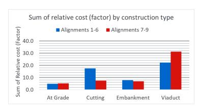
Graph 8: Comparison between Northern (alignment 1-6) and Southern (alignment 7-9) routes by relative cost construction type.
