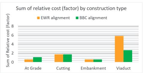
Graph 5: Comparison of relative cost by construction type EWR alignment versus BBC proposal
