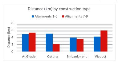
Graph 7: Comparison between Northern and Southern alignments by distance by construction type.
