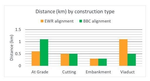
Graph 4: Comparison of distance by construction type EWR alignment versus BBC proposal
